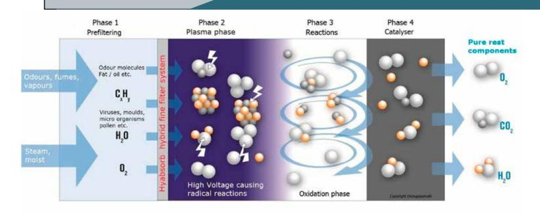
**PHASE 4:** The second stage of the oxidation process in the catalyst removes, based on the longer residence time, the remaining odour molecules
