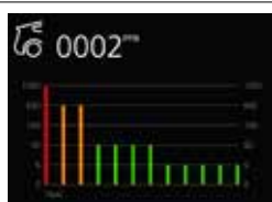
Graph of the concentration of NO 2 detected in the environment.
